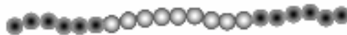
Fig. 5. A schematic presentation of an ABA tri-block copolymer with two A-blocks (gray circles with dark centers) and one B-block (gray circles with light centers)
